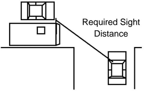
The diagram illustrates the required sight distance between two vehicles on a street. A larger vehicle is on the left, and a smaller vehicle is on the right. A line labeled 'Required Sight Distance' connects the front of the larger vehicle to the rear of the smaller vehicle, indicating the minimum distance needed for the driver of the larger vehicle to see the smaller vehicle in time to stop.
